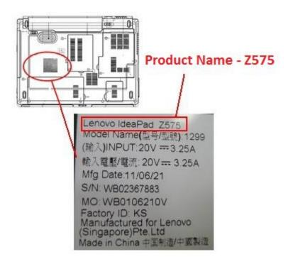
The serial number is printed on the label at the bottom of your machine.
