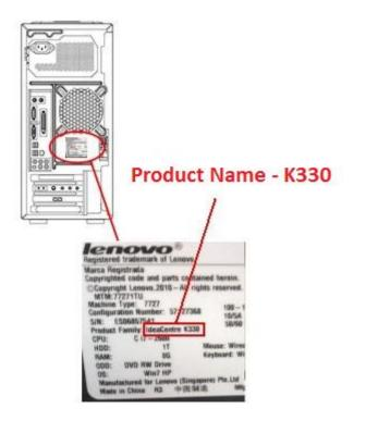
The serial number is printed on the label at the rear chassis of your machine.
