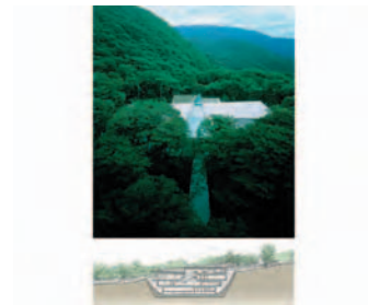
Cross section: The hemispherical substructure was designed to avoid interrupting the flow of groundwater.
