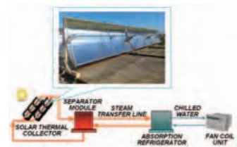
System Flow Diagram of Hitachi Solar Cooling
