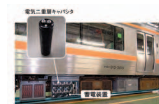
Energy storage system (EDLC): COB015-A0, DC/DC converter system: COV068-A0
