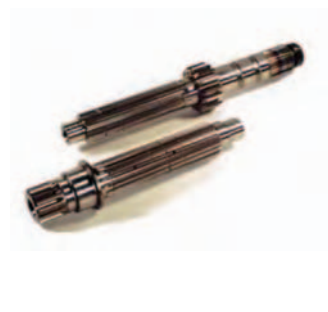
Main shaft (top) and counter shaft (bottom)
